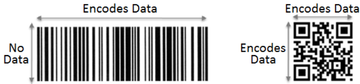
Figure 1. Codes that store data in one dimension (left) and two dimensions (right).
